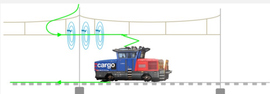
Simplified representation of the detection method of the contact line end by means of the magnetic field.
