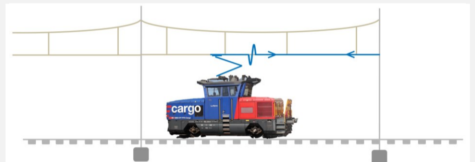
Simplified representation of the method of contact line end detection by means of the high frequency reflection.
