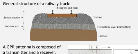
A GPR antenna is composed of a transmitter and a receiver. The former sends a signal downwards. Changes in the material reflect a portion of the signal, which is recorded by the receiver.
