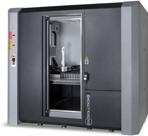
X-ray tomography + in-situ testing and Digital Volume Correlation for cavitation and fracture phenomena or for 3D full-field data collection on different material behaviors
