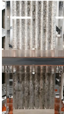
Void-fraction distribution in a fuel bundle using \gamma -tomography
