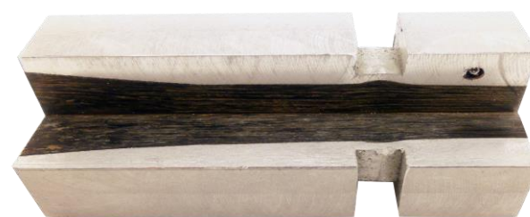
Fig. 3: cut away view of pultrusion die
