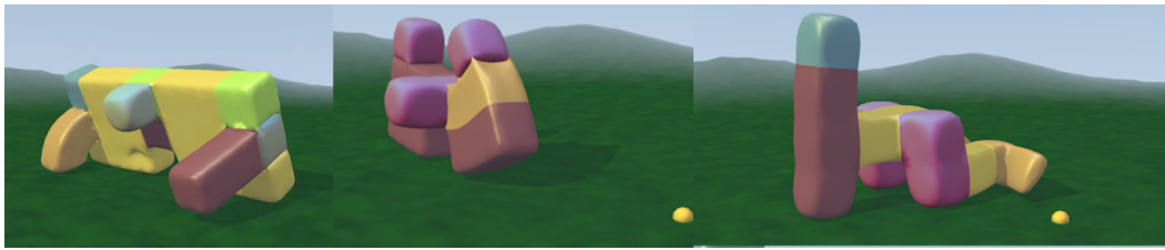
FIGURE A.5: Walking robot designs simulated using position-based dynamics.
