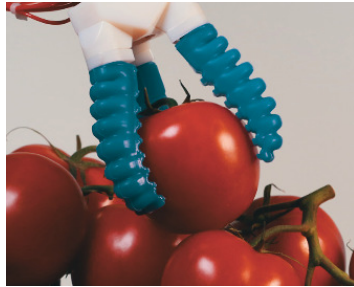
FIGURE 1.1: An example of a soft gripper for food handling, from [15].
