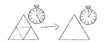
Part consolidation is possible with AM because of the geometric freedom it affords. The construction of complex parts is possible without fear of significant additional costs due to complex geometries, and it is possible to construct artifacts that are not geometrically possible with traditional manufacturing methods. Thus, multiple functions can be condensed into one part.
