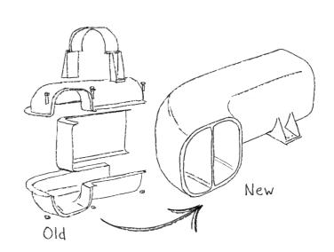
AM allows for customization at low or no additional cost, therefore changes to the geometry of the part can be tailored to the product requirements of each specific artifact.
