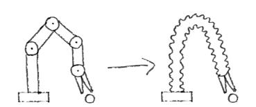
Optimized structural topologies and geometries take full advantage of the geometric freedom allowed by AM. By using the optimized design, artifact mass can be reduced and/or performance can be increased.
