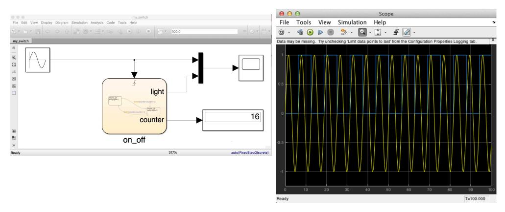
Running the simulation shows a square wave that toggles between 0 and 1 at rising zero crossings of the sine wave
