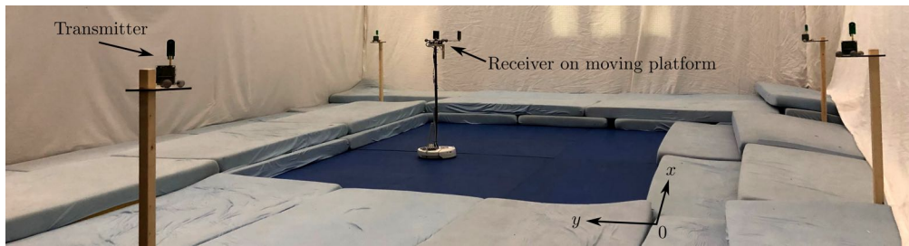
Fig. 6. In order to measure the CIR for different AOAs, different AODs and different distances, a UWB receiver is mounted on a moving, rotating platform (Roomba). Transmitters send signals in a random fashion to the receiver, which measures the associated CIR. Both receiver and transmitter are equipped with markers which can be seen by the overhead motion capture system for purposes of gathering ground-truth data.
