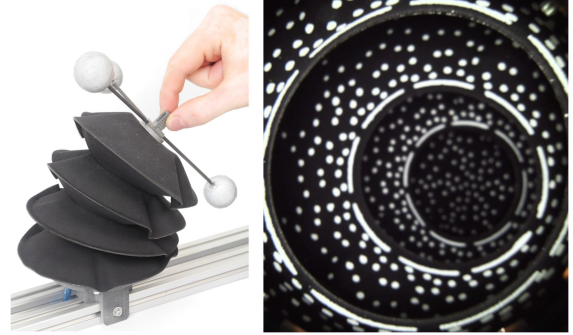
Fig. 1. Left: A linear soft inflatable bellow actuator with an integrated camera is manually deflected. Markers for an external motion capture system are mounted on top and are used as ground truth during training. Right: Image recorded by the internal camera showing the pattern employed in white. The proposed sensing approach predicts the tip position of the actuator (located on the grip) using only images from the internal camera.
