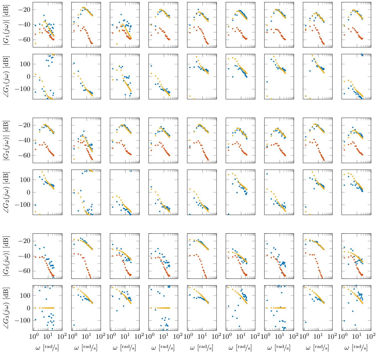
Figure 1: Estimated transfer function (blue) from the inputs to the angular rates ( $\omega_x$  top,  $\omega_y$  middle,  $\omega_z$  bottom). The fit resulting from the augmented model is shown in yellow and the standard deviation is indicated in red.
