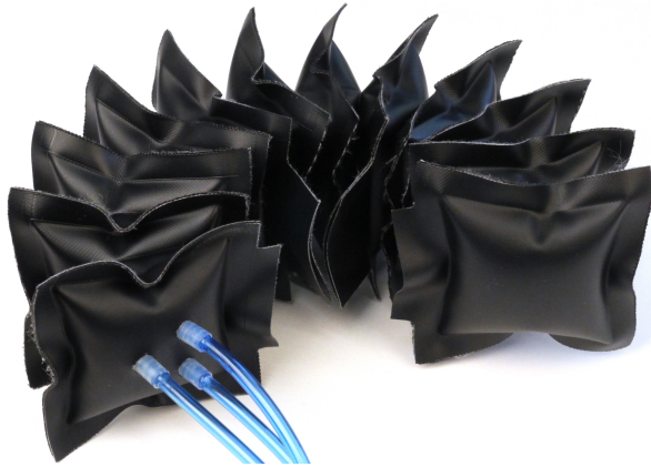
Fig. 2. The bellow-type actuator made from polyurethane coated nylon in fully inflated state. The actuator consists of twelve single cushions and the front side measures 100 \times 100 mm in a deflated state. When fully inflated, the maximum actuation range, is approximately 190^\circ . Two tubes connect the actuator to the control valves, while the third one is used to measure the pressure in the actuator.
