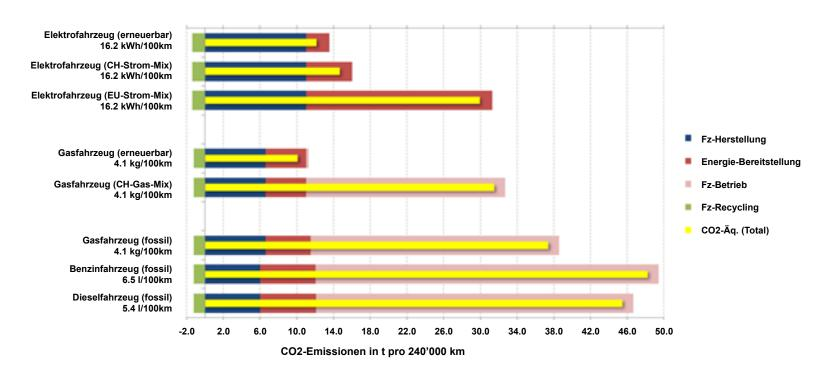
Source: Bauer et al, Applied Energy (2015), Fuchs et al. ATZ (2014), Audi (2015), fuel consumption from Spritmonitor.de for VW Golf 81-85 kW (MJ 2014/2015). Biogas according to LCA-Study Empa-PSI-Agroscope-Doka (2012); EU-Strom-Mix: 522 g CO<sub>2</sub>/kWh, CH-Strom-Mix: 130 g CO<sub>2</sub>/kWh, renewable Electricity: 65 g CO<sub>2</sub>/kWh
