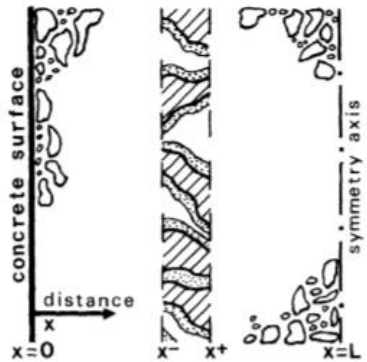
Figure 4. Slab and control volume geometry.
