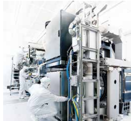
An ASML NXE:3300 EUV scanner under assembly.
