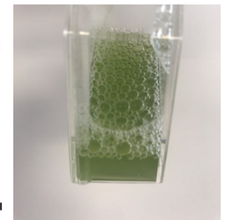
Cyanobacteria producing 1-butanol from solar energy and CO 2
