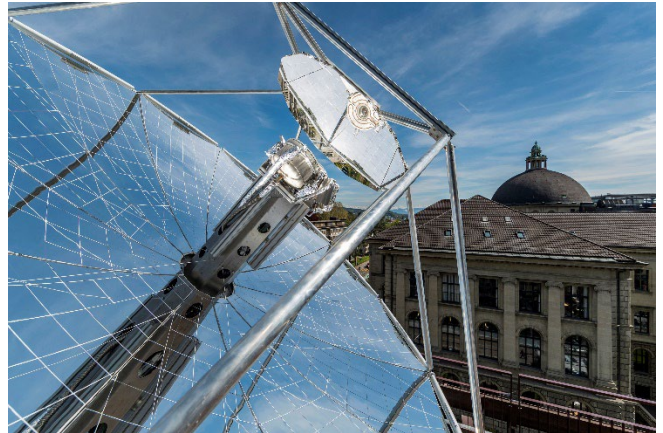
Fuels from Sunlight and Air – The solar mini-refinery mounted on the roof of ETH Machine-Laboratory demonstrates the entire process chain to carbon-neutral fuels. Using concentrated solar radiation, a high-temperature solar reactor splits CO 2 and H 2 O extracted directly from ambient air and produces syngas – a tailored mixture of H 2 and CO – which is finally processed into drop-in hydrocarbons such as methanol or kerosene. These transportation fuels are carbon neutral because solar energy is used for their production and because they release only as much CO 2 during their combustion as was previously extracted from the air for their production. In particular, solar kerosene can contribute towards making long-haul aviation sustainable.
