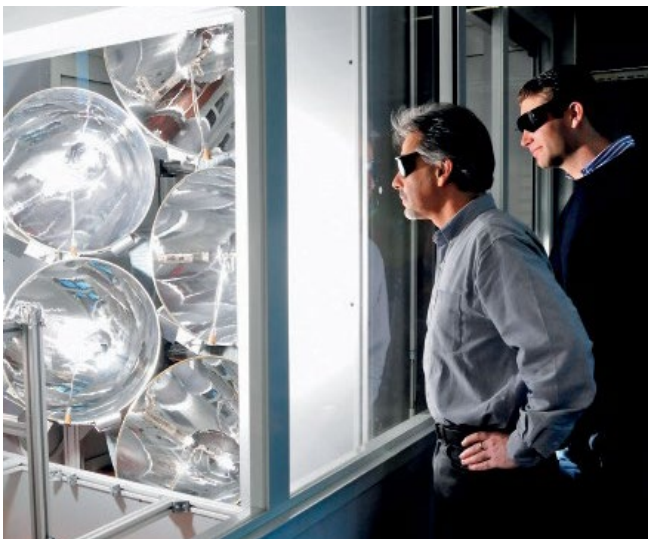
Experimentation at the High-Flux Solar Simulator – Solar thermal receivers and thermochemical reactors are subjected to high radiative fluxes ( > 5,000 suns), and tested at high temperatures ( > 1000^{\circ}\text{C} ) and heating rates ( > 1000^{\circ}\text{C/s} ), mimicking the radiative heat transfer characteristics of highly concentrating solar systems.
