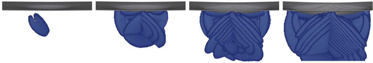
Figure 18.8: QC Simulation of 3D nanoindentation with a spherical indenter (radius 40 nm) into single-crystalline (100) Cu up to a penetration depth of about 3 nm, for details see [3]. Images adapted from reference [47].
