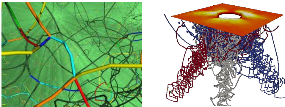
Figure 20.1: Two examples of Discrete Dislocation Dynamics, highlighting a collection of discrete dislocation line segments within a crystal treated as an elastic continuum (the left image is adapted from ParaDiS [7], the right image from TRIDIS [80]).
