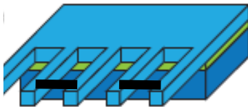
Scheme of CNTs (black line) grown on MEMS structures dedicated for dry CNT transfer into future devices.
