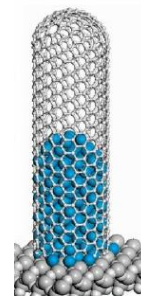
Illustration of a SWNT growing from a metal catalyst (image: S. Hofmann et al.: Nano Letters, 7 (2007) 602).
