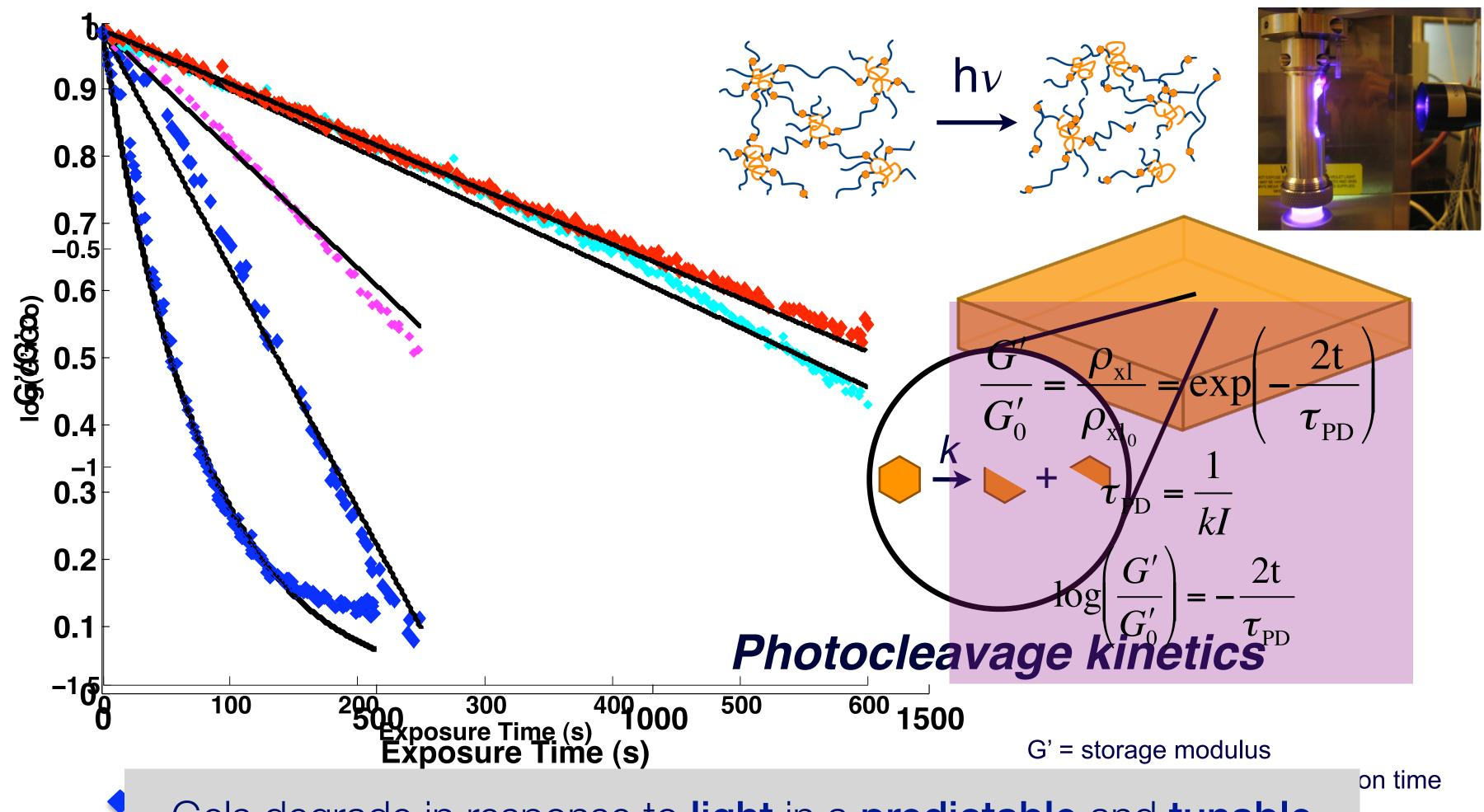
Gels degrade in response to **light** in a **predictable** and **tunable** manner that is quantified with a **statistical-kinetic model**.
