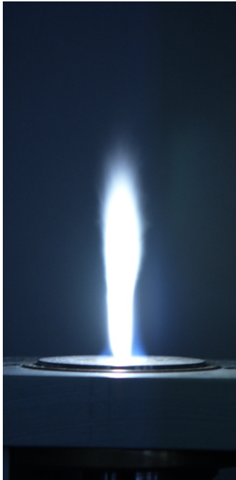
Spray flame producing Pt/Al 2 O 3
