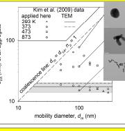
**Figure 3:** The  $d_{VA}$  of Ag nanoparticle agglomerates generated by Kim et al.<sup>4</sup> is obtained by the proposed equation and compared to particle diameters  $d_p$  obtained by TEM<sup>4</sup> (grey area represents standard deviation of  $d_p$  at T = 293 K). Higher furnace temperatures (T = 473 – 873K) lead to faster sintering and larger  $d_{VA}$ .
