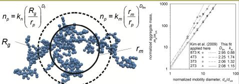
**Figure 5:** The DMA-APM data of silver nanoparticle aggregates sintered at different temperatures by Kim et al.<sup>4</sup> are post-processed here. The  $D_{fm}$  exhibits a monotonic increase consistent with our sintering simulations (Fig. 4).
