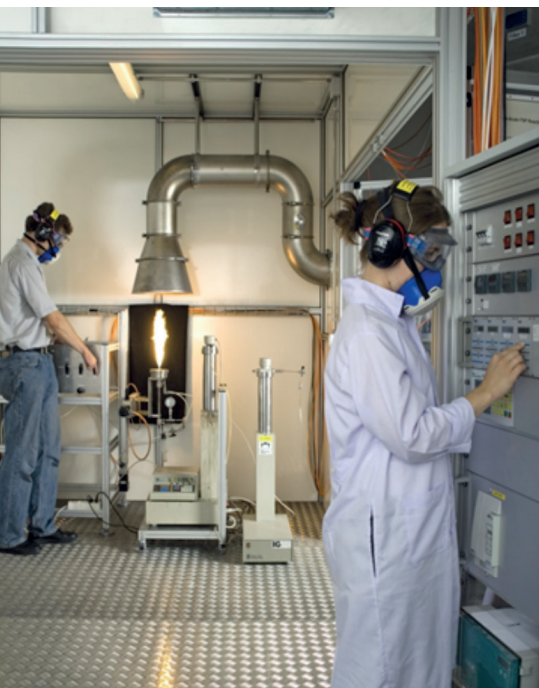
Production of nanoparticles with flame spray pyrolysis.
