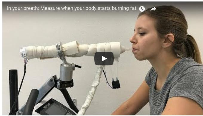
Blow into the tube, please. In the future, the procedure will not just be used by police checking for alcohol intoxication, but also for testing the condition of athletes and for people who want to lose that extra bit of weight. A sensor developed by ETH researchers makes it possible to measure when the body starts burning fat with a convenient breathalyser.
