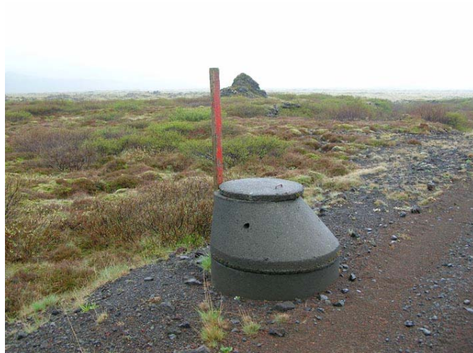
A research well (No° NL-3) between in the lava field Hagavíkurhraun between Lækjarhvarf and lake shore.
