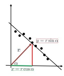
$$\frac{\partial S(r,\alpha)}{\partial \alpha} = \frac{\partial}{\partial \alpha} \sum_{i} (x_c \cos(\alpha) + y_c \sin(\alpha) - x_i \cos(\alpha) - y_i \sin(\alpha))^2$$
