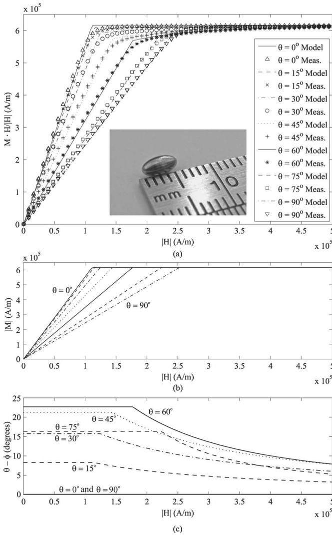
Fig. 2. Modeled and measured magnetization versus applied field strength for various applied field angles. (a) Experimental data of the component of the magnetization parallel to the applied field. (b) Inset shows the machined ellipsoid used in the experiments. The magnitude of magnetization predicted by the model. (c) Angle between the applied field and the predicted magnetization.
