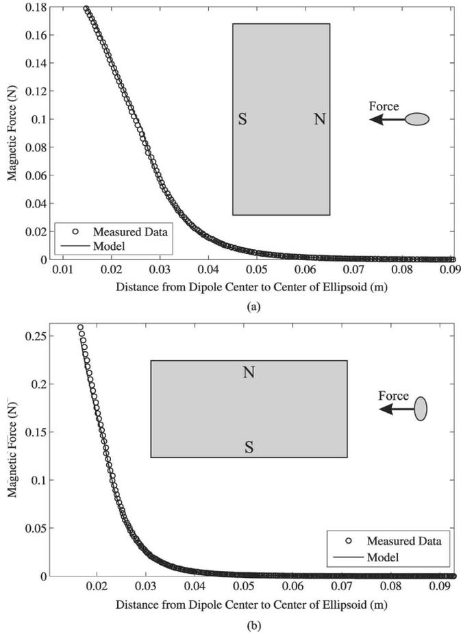
Fig. 5. Modeled and measured force magnitude versus distance from the dipole center, which lies below the magnet’s surface. (a) Axial direction. (b) Lateral direction. The insets illustrate the experimental setup, drawn with a 1:1 scale to the data. The left edges of the plots correspond to the surface of the magnet.
