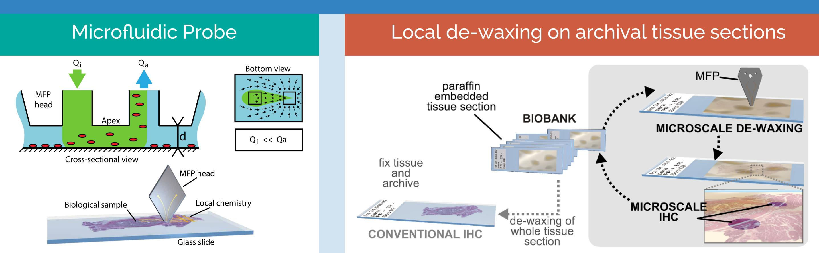
The microfluidic probe (MFP) is a non-contact, scanning technology that operates in the "open-space" [1]. The MFP allows to perform chemistry on surfaces at the micrometer length-scale by hydrodynamically confining a processing liquid within an immersion liquid [2-3].
