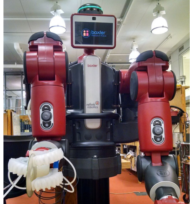
Fig. 1: The soft robotic hand, mounted to the wrist of a Baxter robot, is picking up a sample object.
