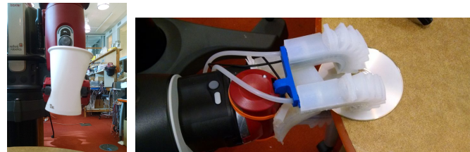
(a) Cup squashed (b) Gripper performs a compliant grasp to pick up a thin object off a table.
