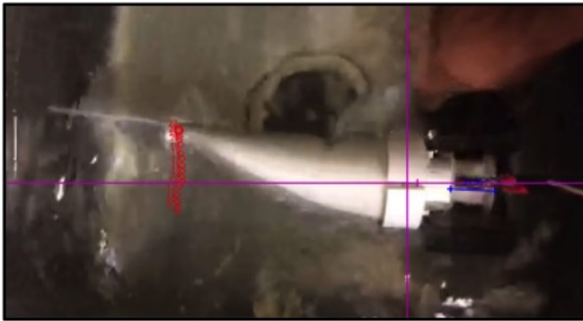
Fig. 11: Tracking Analysis of the test body flexion utilizing the new brushless external gear pump at 0.9 Hz. The end of the test body is tracked in each frame. Its angle with respect to the origin (purple lines intersection point) is calculated and used as the measurement of body deflection.
