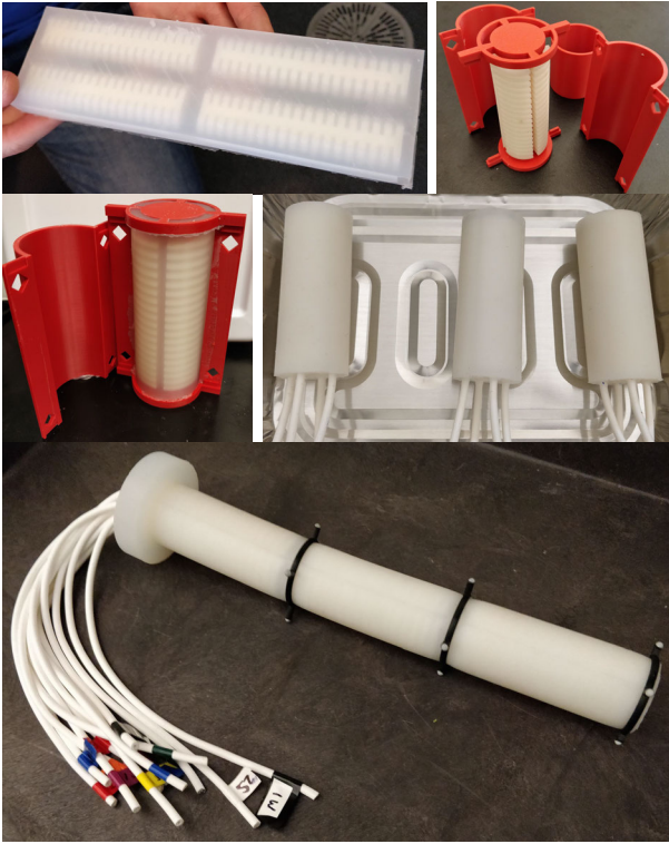
Fig. 8. Overview of the Manufacturing of the 3D Soft Arm Prototype. From Top Left to Bottom Right: Creation of four wax cores through casting; assembly of wax cores into 3D printed molds; casting of Silicone Rubber into the mold; Removal of wax through melting and addition of silicone tubing; Routing of tubing, gluing, labeling and adding markers.
