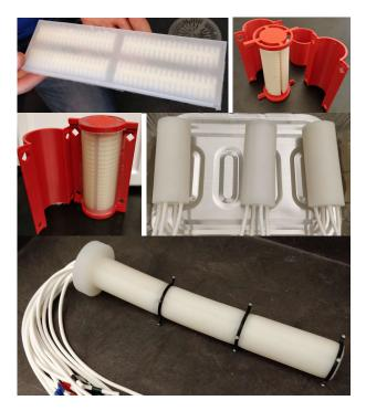
Fig. 10. Manufacturing overview of the 3D soft arm. From Top Left to Bottom Right: Creation of four wax cores through casting; assembly of wax cores into 3D printed molds; casting of Silicone Rubber into the mold; Removal of wax through melting and addition of silicone tubing; Routing of tubing, gluing, labeling and adding markers.
