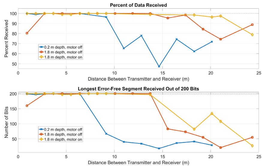
Figure S16: Acoustic range tests. Results of transmitting a sequence of 200 alternating bits at 20 bits/s at various depths and distances, in order to characterize the acoustic communication performance.
