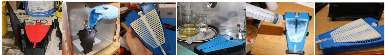
Figure S9: Wax core fabrication. Fabrication steps from left to right: 3D print model core; Create silicone mold; Release model core; Heat beeswax and mold; Pour wax with syringe; Demold wax core.
