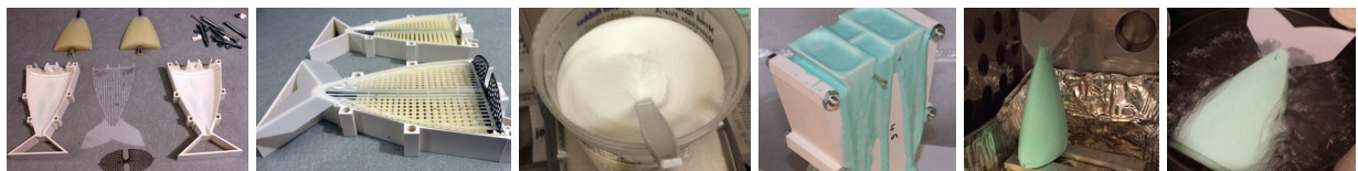
Figure S10: Tail fabrication. Steps from left to right: Assemble individual parts of the tail mold; Mix silicone rubber and glass bubbles; Degas and cure silicone rubber fish tail; Melt out the wax core in an oven; Remove residues of wax with hot water bath.
