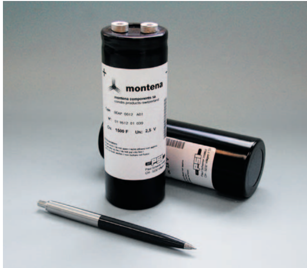
Fig. 4.2-4: Supercapacitors reach an unprecedented high capacitance of thousands of Farad by increasing the electrode surface of traditional electrolyte capacitors (with about 0.01-0.1 Farad) by factors of up to 100 000. This is achieved by using coal particles with surface properties that can be described by applying the concept of fractal geometry (surface dimension of the electrodes is about 2.6). 100 elements with 2700 Farad and a maximum of 2.6 Volts are sufficient to provide 30 kW for 20 s, and to accelerate, e.g. a 1000 kg car to 120 km per hour. If combined with fuel cells producing continuous power of only 30 kW, a car with good dynamical properties results without the fuel cell stack being oversized (for the sake of acceleration, today's car engines are oversized by a factor of 2 to 8).
