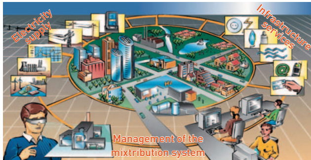
Fig. 4.3-3: High integration of information and communication electronics with power electronics contributing to mixtribution in the future. Decentralized electricity generation (e.g. photovoltaics, fuel cells, wind power, small co-generation units) combined with larger generation capacities will be managed as virtual power plants including real time electricity prices for small consumers operating automatised electrical appliances
