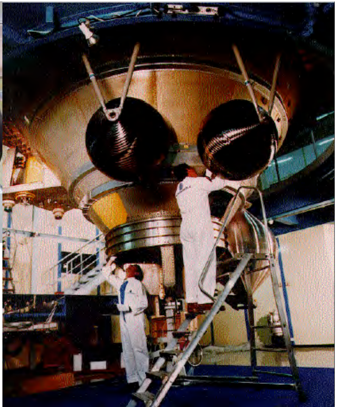
Figure 1: Ariane 5 composite high pressure tanks
