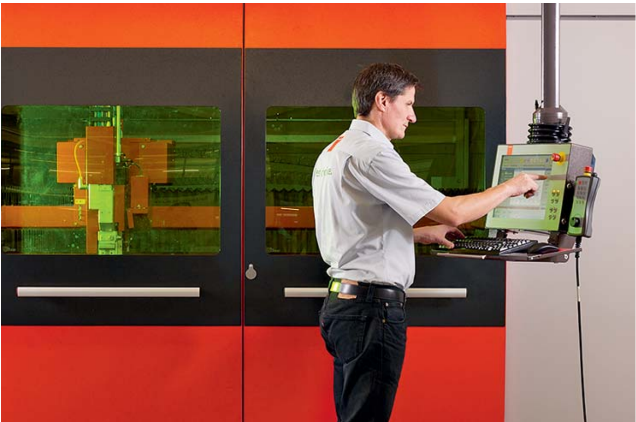
Figure 15: A laser product in a manufacturing area is equipped with a protective housing that provides complete shielding.
