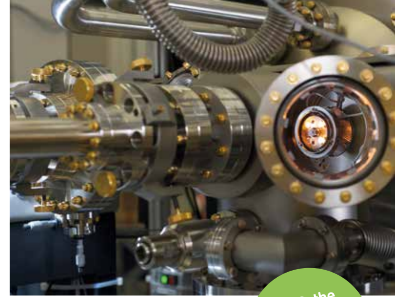
Close-up showing the buffer chamber of a molecular beam epitaxy apparatus with transfer rod (horizontal) and heating station (glowing orange) for probe cleaning. Tubes (top) provide the liquid nitrogen that cools parts in the growth chamber (Wegscheider group, ETH Zürich).
