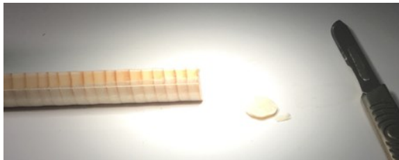
Fig. 1: A scalpel was used to divide the individual tree rings into two early-wood and one late-wood fraction.
