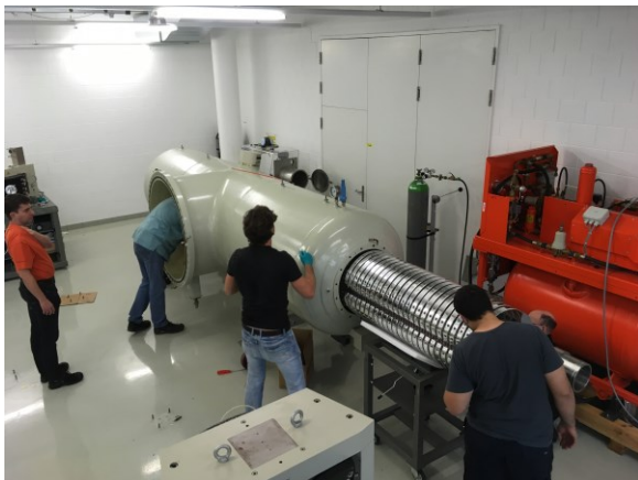
Fig. 1: Removing the acceleration column out of the tank for complete disassembly at La Chaux-de-Fonds.
