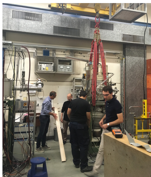
Fig. 2: Moving the 0^\circ ion source to its new (original) position.
