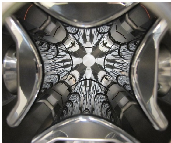
Fig. 1: The new quadrupole focusing system (view along the beam axis) [2]. Its main purpose is ensuring optimal ion optics for all charge states and isotopes.
