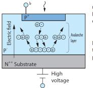
Generated carriers produce new electronhole pairs while being accelerated by high electric field. Ionization
