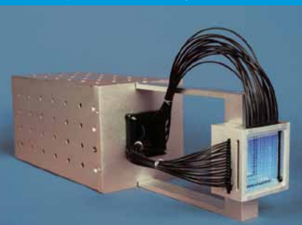
Beam profile monitor with orthogonal fiber ribbons
