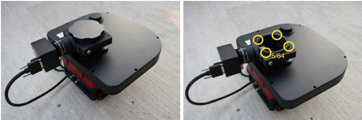
Figure 43: SBIG camera with attached filter wheel. For storage attach the cover plate ( top ). For mounting the camera loosen all four 5/64" Allen screws at the camera flange.
