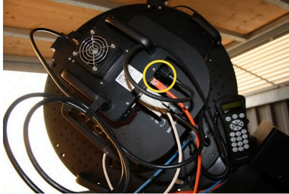
Figure 42: Attach the camera power cable and the USB cable. Note: in this image instead of the USB cable the Ethernet cable is used. However, only use the USB-cable!
