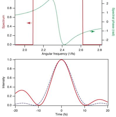
Temporal FWHM of pulse with nonlinear spectral phase is shorter than "transform-limited" pulse
