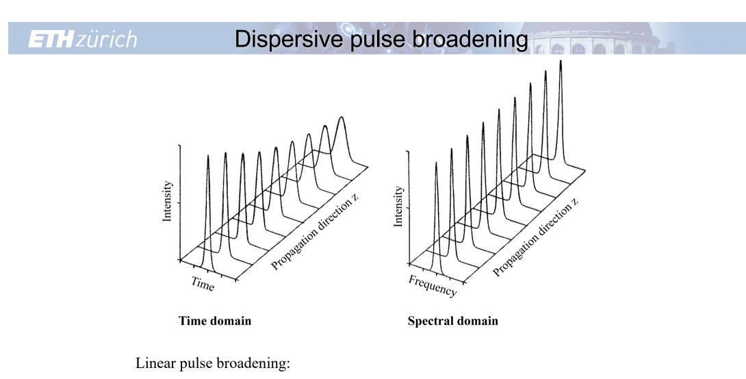
Transform-limited pulse is broadening in the time domain but its spectrum remains unchanged.
