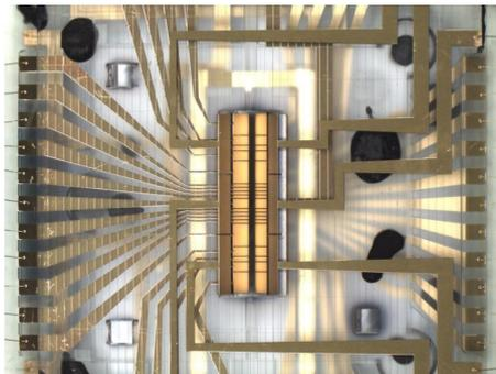
Figure 3.2: The Weizmann trap, the ion trap used for experiments in this thesis. Figure adapted from [45].
