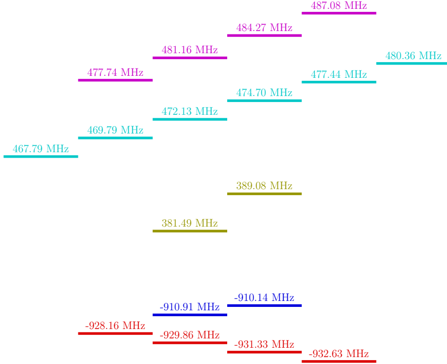
Figure 2.2: Schematic representation of the hyperfine states of the ortho-groundstate (\nu, L) = (0, 1) at 450 \mu\text{T} . Colors represent different (F, J) quantum numbers, with corresponding hyperfine energy levels labeled in MHz. Horizontal positions indicate different M_J values, ranging from left (negative) to right (positive). Note that these states are the eigenstates of the Hamiltonian rather than the pure |F, J, M_J\rangle states. The figure is illustrative and not to scale.
