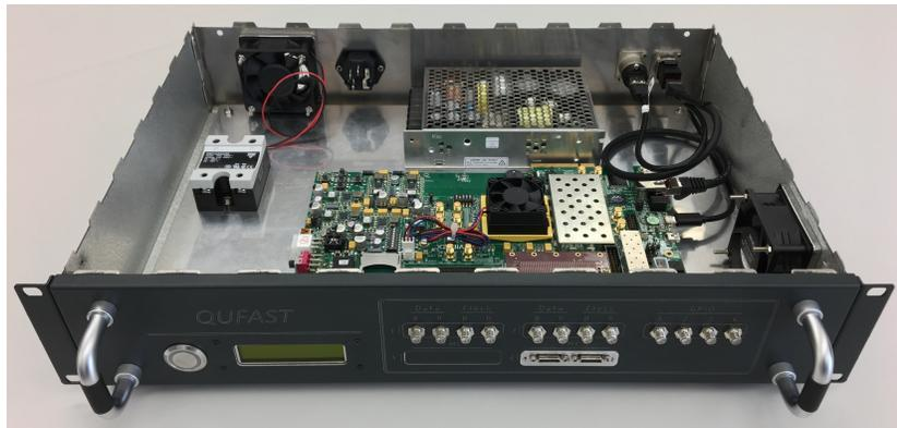
Figure 2.3: Preliminary layout of the enclosure containing the FPGA and frame grabber board. Shown is the front view without the top lid. The front panel features 12 SMA connectors, one FMC422 board, a user controllable LCD screen and a power button. Inside it hosts the VC707 evaluation board, a power supply (240 V to 12 V, 100 W Max.) and a relay. On the back, there are power, USB and Ethernet feedthroughs. Fans on the side and back provide airflow for cooling.
