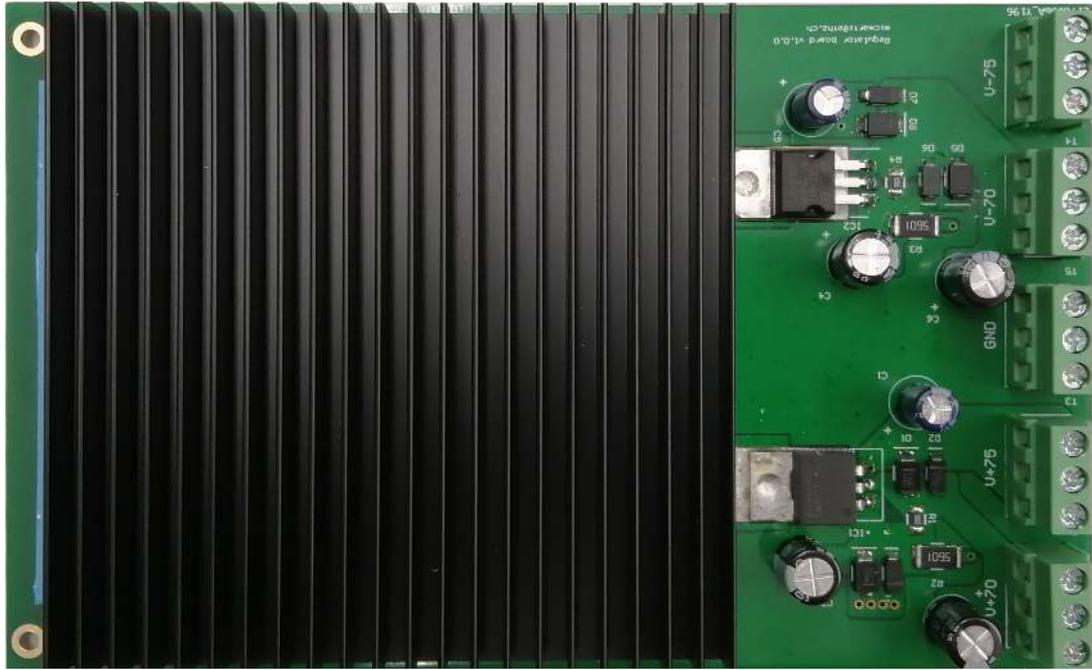
Figure 3.13: Image of the regulator board. As with the amplifier board, power connectors are screw terminals. Otherwise, the board is mostly a heat sink for the three-terminal regulators.
