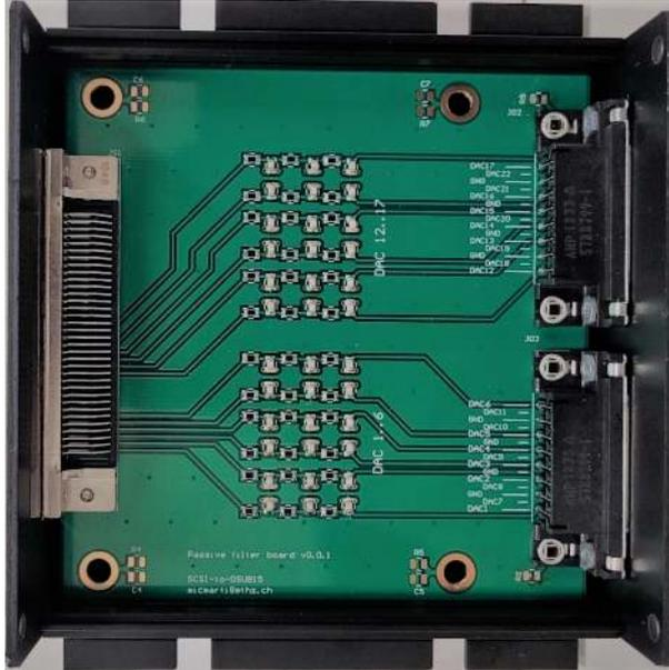
Figure 4.3: Passive filter board fitted into an enclosure.
