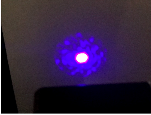
(a) Degraded PCF spot as seen on a card inserted after the collimator.
