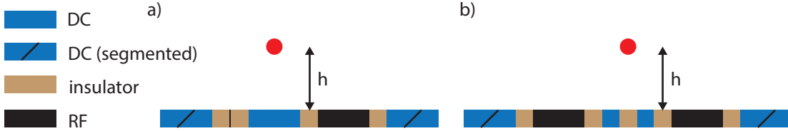
Figure 2.2: The electrode arrangement of an SET. The ion position (pseudopotential minimum) is shown in red. The confinement in the plane out of the image is obtained by DC voltages applied to the segmented electrodes. (Left) Five-rod configuration. (Right) Six-rod configuration. Both configuration allow for multi-zone operation without segmenting the middle electrode(s).
