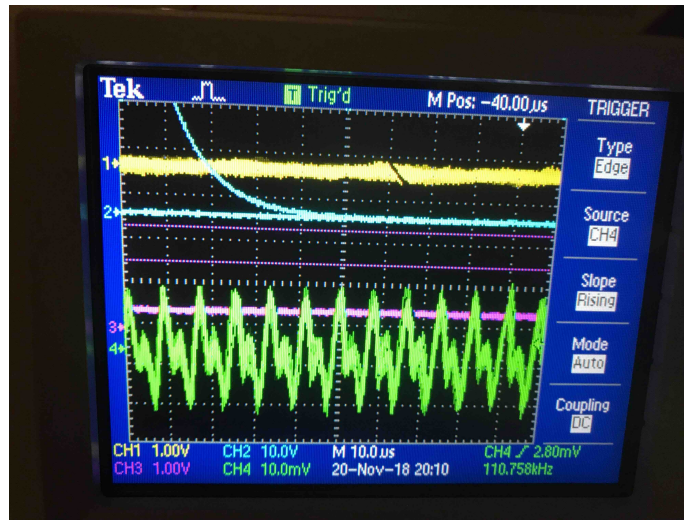
Figure 4.15: Photo of a typical TA output ripple as seen on the oscilloscope (green trace). The TA output is attenuated and sent of a PD, which is AC-coupled on the oscilloscope.
