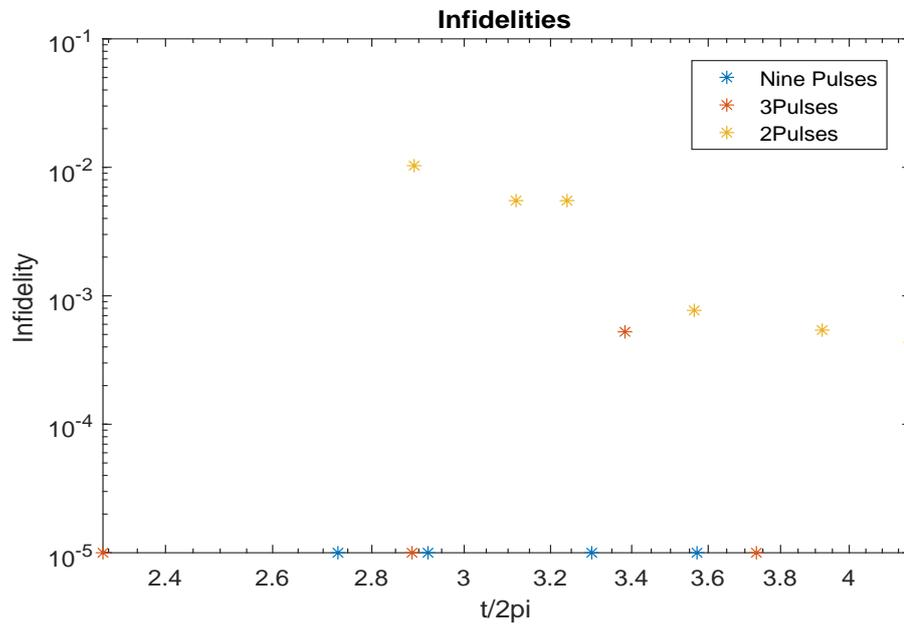
Figure 4.4: We have compared the fidelity that can be achieved using sequences made by a different number of pulses when we include at the first order both centre of mass and stretch mode, without the carrier. As we can see, three pulses are enough to achieve  $IF = 1 \cdot 10^{-5}$ .
