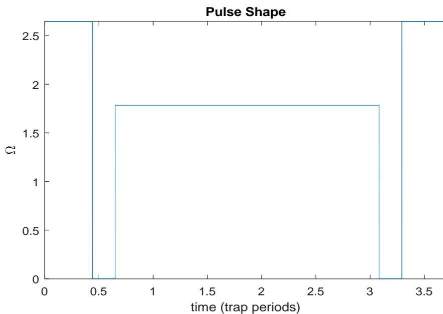
Figure 4.2: Symmetric series of three pulses. On the  $x$  axis we have the time of the gate express in COM mode periods.
