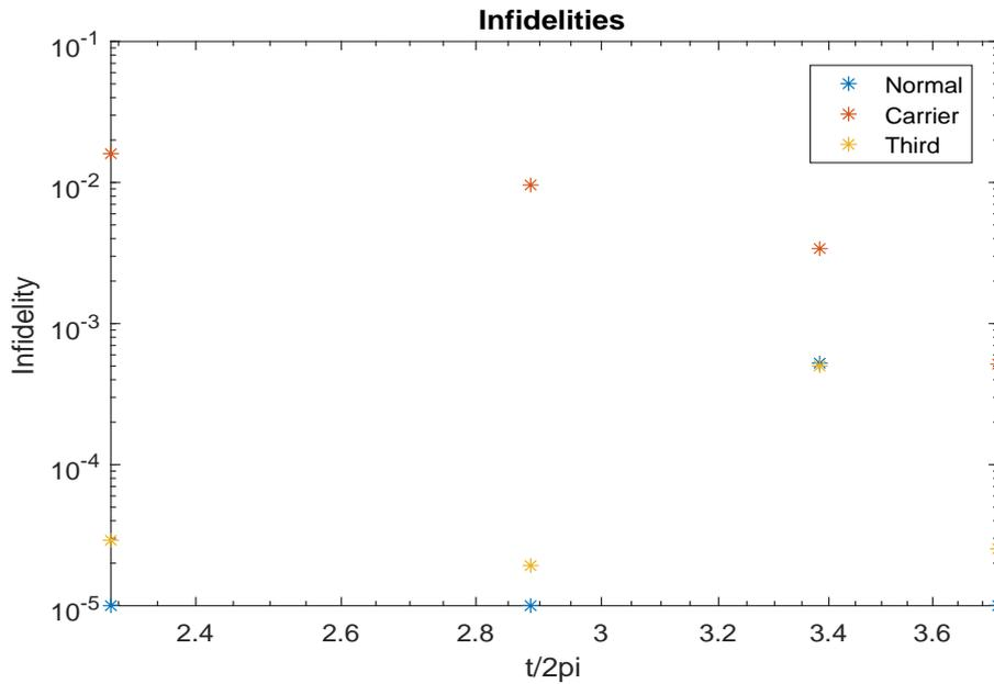
Figure 4.1: We have analysed the effect that a small carrier term (red) and the third order terms (yellow) can have on the achievable fidelities of our gate. In particular, we can see that the small carrier term caused by an imbalance in the laser beam, can considerably influence our precision, increasing the infidelity of 3 orders of magnitude.
