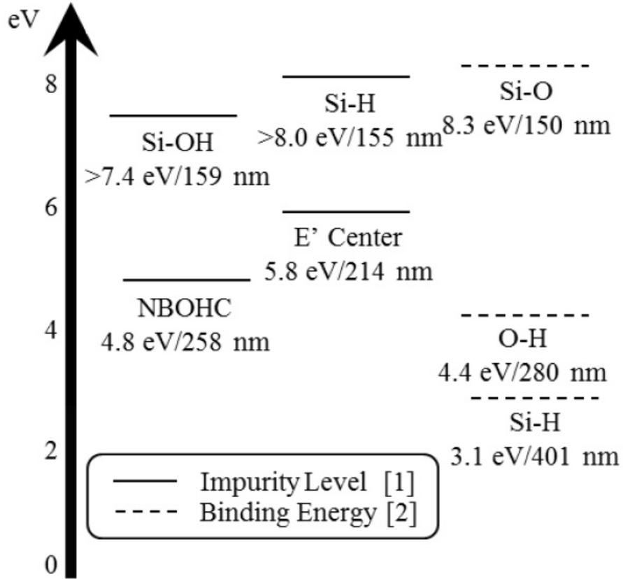
Figure 1: This diagram shows the impurity levels and binding energies of certain of E' and NBOH centers and their products after reacting with the hydrogen (Si-H and Si-O-H) [4].
