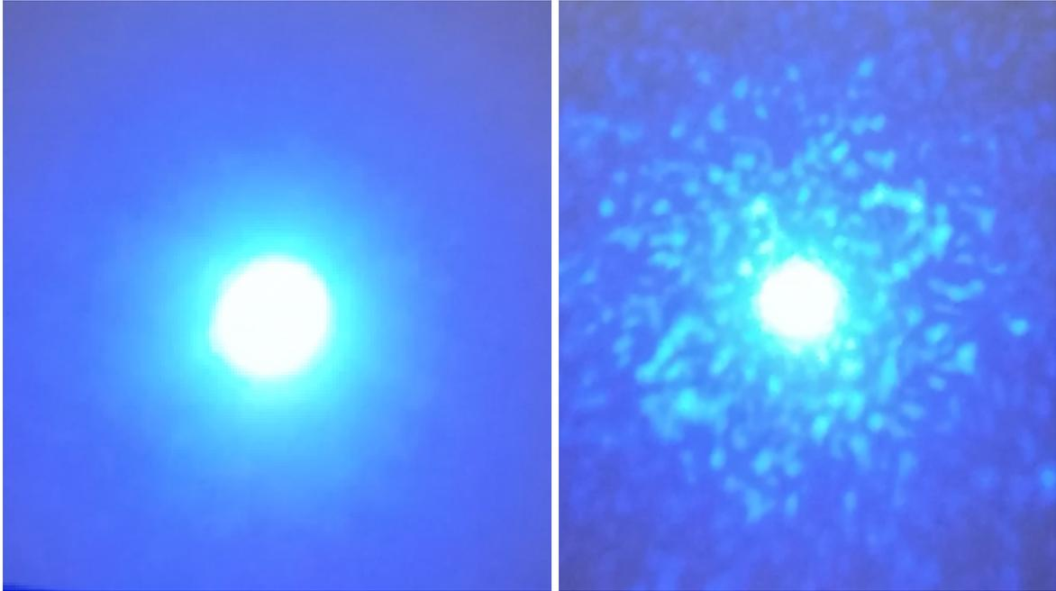
Figure 4: This figure shows both the output beam of the fiber that has been cured for 24 hours before the transmission drop (*left panel*) and after 77 hours at 140°C (*right panel*).
