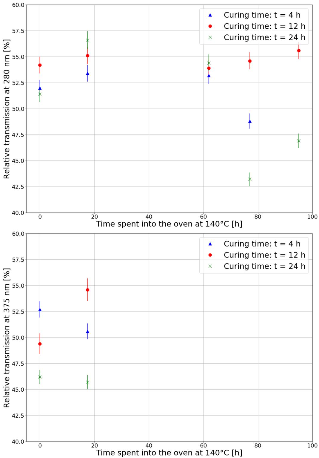
Figure 3: Transmission at 280 nm (*upper panel*) and 375 nm (*lower panel*) for three fibers cured at 250 mW with a 313 nm laser for different time spent into the oven.
